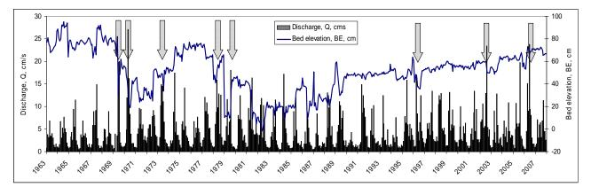
Figure 8. Temporal changes in mean bed elevation superimposed on peak discharge values for the Suceava River, Brodina gage station.
