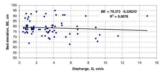
Figure 10. Relation between the height of the river bed (BE) and the size of the liquid flow (Q) at the Brodina hydrometric station, the Suceava River.
